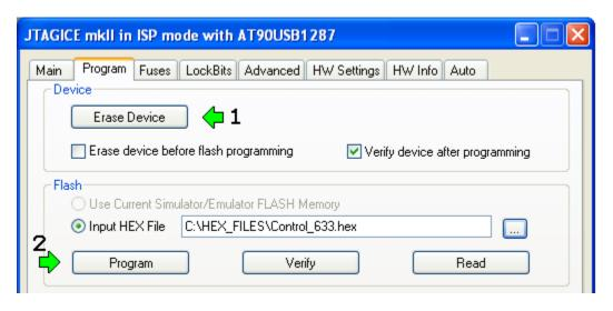
You can monitor the progress by watching the progress bar in the main application. The progress bar will make two passes: once for the programming and once for verification.
