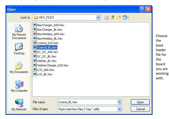
Then press the Program button to load the bootloader. Do not press the Erase Device button!
