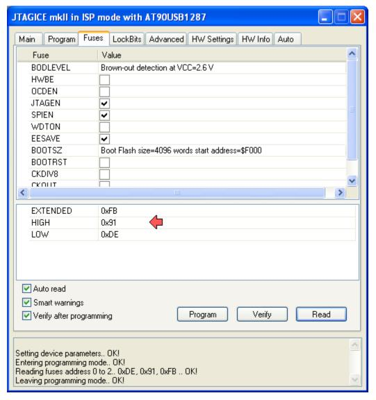
You do not need to check the checkboxes to make changes; just enter the values directly as shown below.
