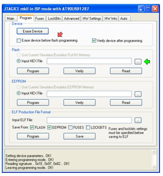
Then press the file locator button under the *Flash* groupbox.
